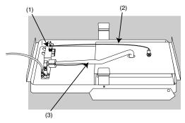
Make sure wire is connected between igniter and electrode. Check that igniter lock nut is tight. *Note: If the igniter works loose, carefully tighten the igniter lock nut with an adjustable wrench or pliers.* Adjust igniter electrode to burner. Gap should be 1/8 to 3/16 inch from tip of electrode to burner. Spark should be a white/blue color, not yellow.
